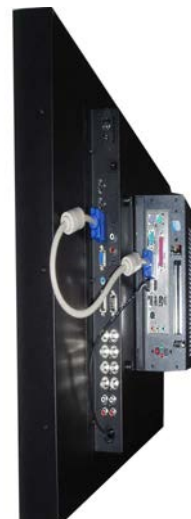
Mini-IPC mounted on Back-Site
