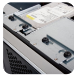
Anti-vibration drive cage design
