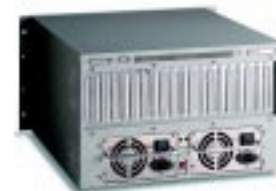
Redundant Power Supply
