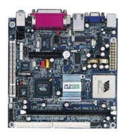
Socket 370 Mainboard with onBoard mounted VIA C3 CPU/ 1000 MHz
