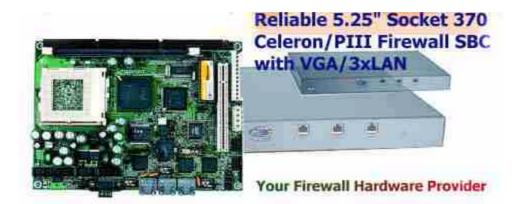
5.25" Celeron/PIII Firewall SBC with VGA / 3xLAN. This board is a very reliable Embedded SBC of firewall for protecting your servers or PCs. It is also suitable using in Network Applications and Server Application as well.
