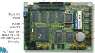
32-bit Digital IO 2½" HDD Interface + power
