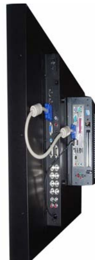
Mini-IPC mounted on Back-Site
