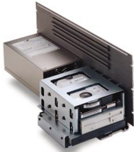
Drive assembly with one slim CDROM drive and two 3 1/2" drives
