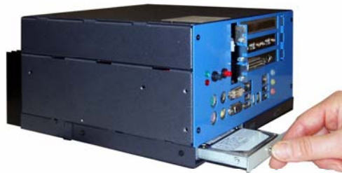
Removable Frame on Mini-IPC - 3 PCI
