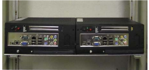
2 Units in a 19" Rack – 2 Height Units
